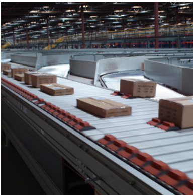
High throughput sortation systems are used by retailers to distribute goods to stores
