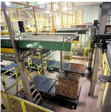
Manufacturers sort by product to feed robotic palletizing cells
