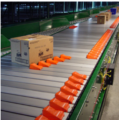
Sliding shoe sorter is an example of a linear sorter
