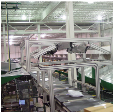
Bar code scan tunnels can read one or multiple sides of cartons and bags on both linear and recirculating sorters
