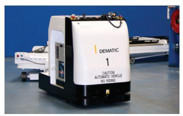
The Compact Tuggers at AER use laser navigation to move throughout the facility, increasing safety for personnel while reducing product and equipment damage.
