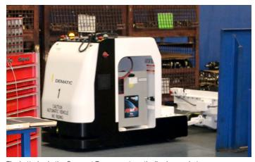
The batteries in the Compact Tuggers automatically charges between new transport requests, so operators don't waste time having to change batteries.
