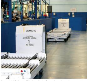
Dematic AGVs at AER Manufacturing automatically transport and deliver engines from production areas to shipping.
