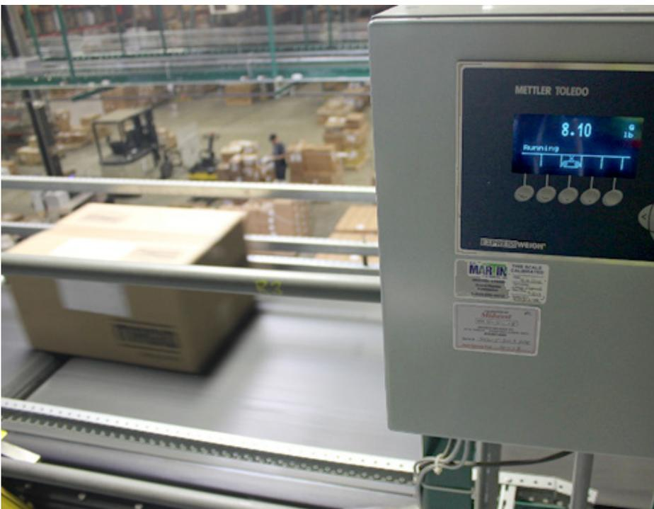
The in-line scale weighs each carton on-the-fly.
