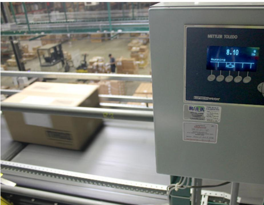
The in-line scale weighs each carton on-the-fly.
