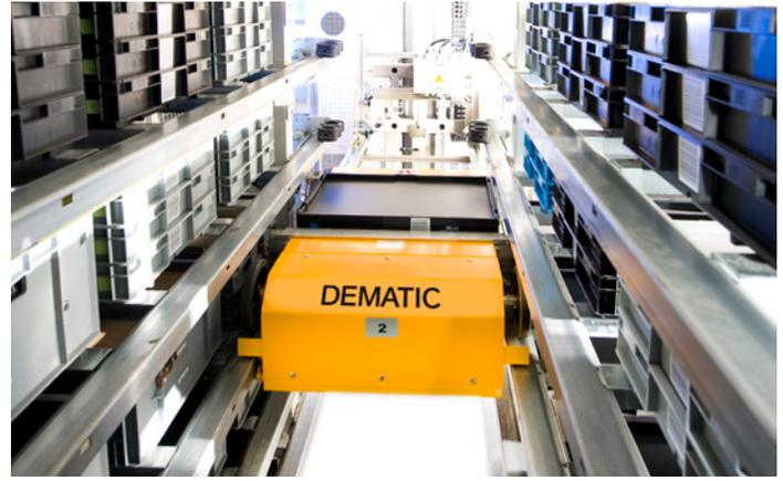
**Multishuttle Work-in-Process Buffer:** Inventory totes are stored in this Multishuttle sub-system until needed at assembly workstations.
