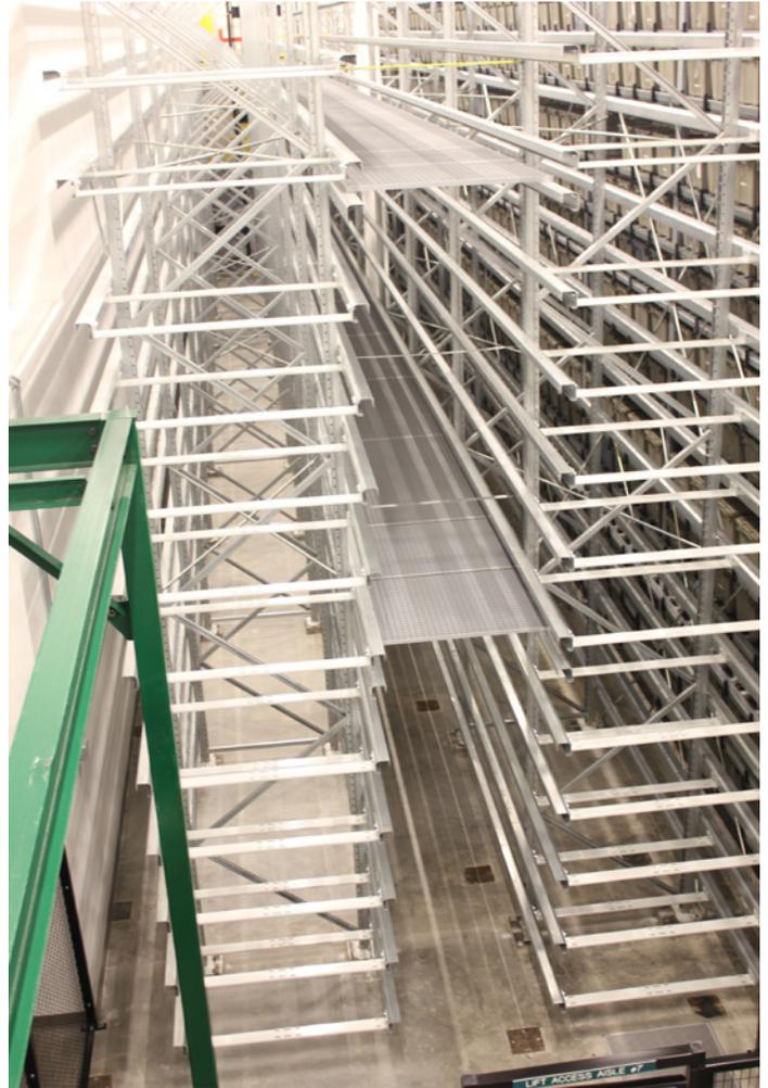
**Future Growth:** Multishuttle racking set up for planned future expansion. The modular design and scalability of the Dematic system allows capacity to be easily added.
