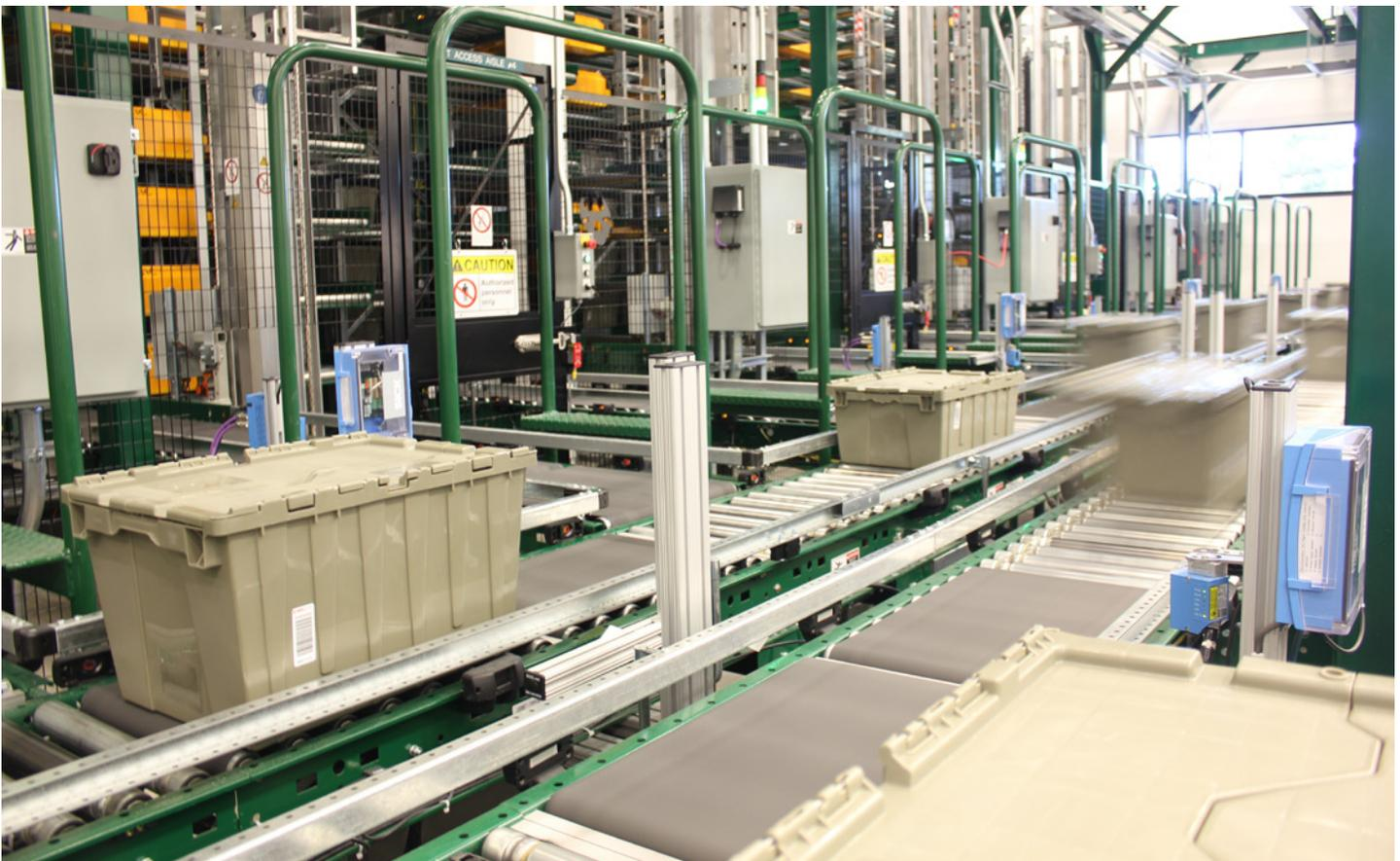
**Multishuttle In/Out Conveyor Loop:** Connects the Multishuttle to the workstations. Inventory totes are brought to and from workstations.
