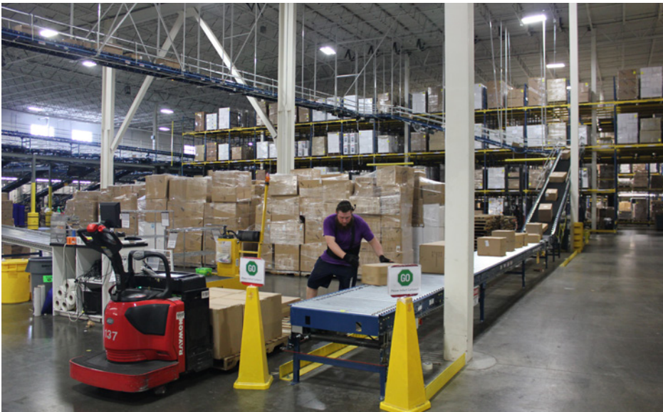
Cartons of product are picked from pallet racking in the warehouse and transported via pallet truck. A distribution center employee inducts the cartons onto the conveyor system.
