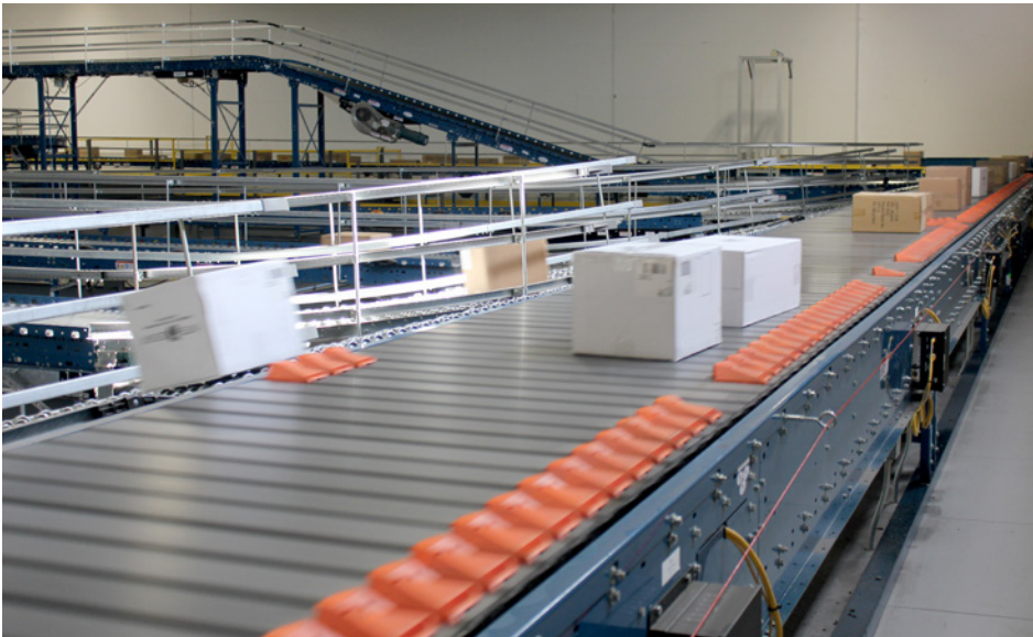
The sliding shoe sorter diverts cartons to the appropriate shipping door.
