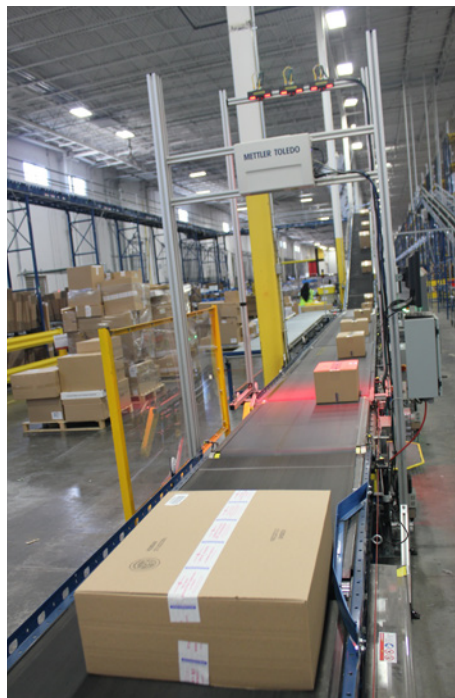
In line scale weighs each carton “on the fly”. A dimensioning scanner provides carton length, width, and height.
