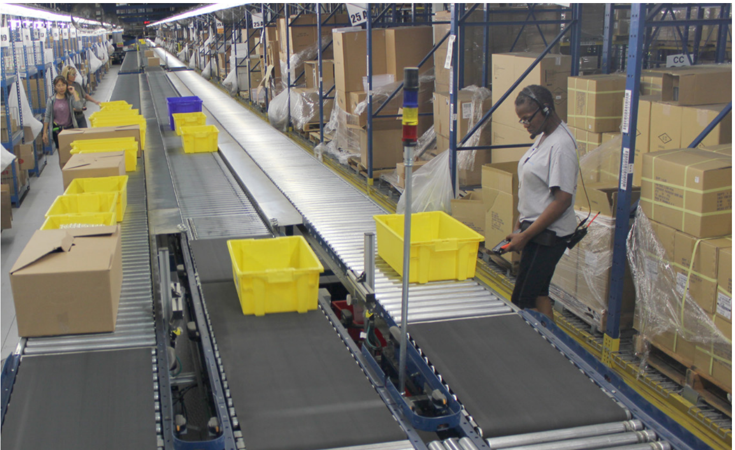
Order totes are automatically diverted from the center conveyor to a side conveyor spur if there are picks in the zone.
