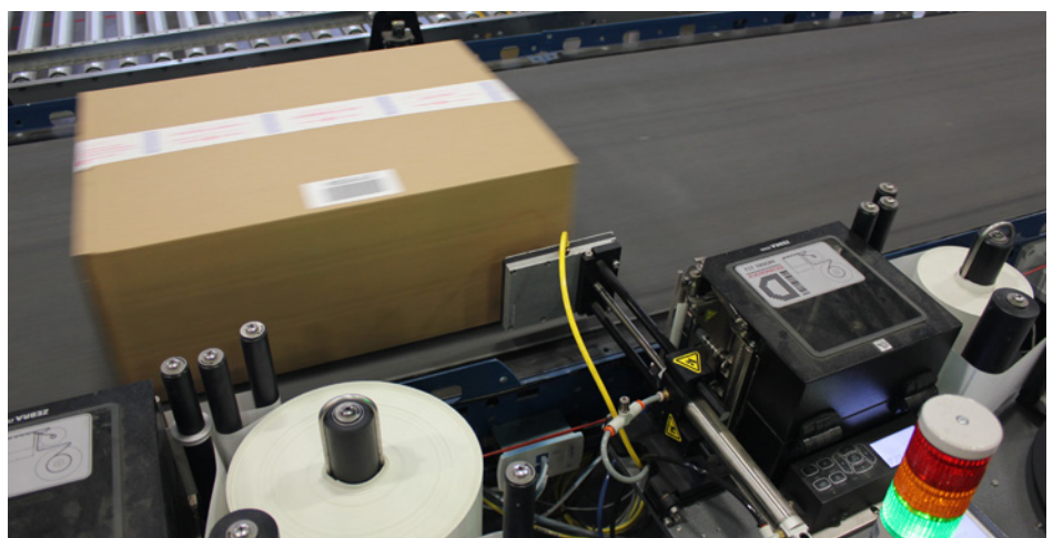
The automatic label print and apply technology is integrated into the conveyor network and control system.
