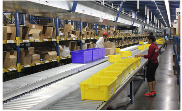
Piece pick items are placed into the order totes on level one of the pick module.
