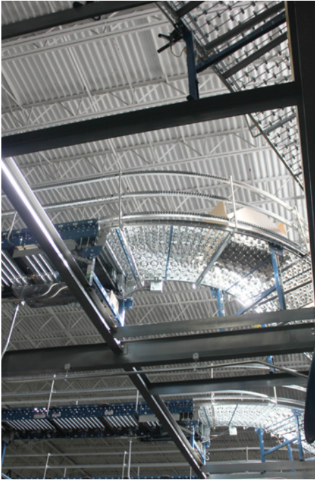
Take-away conveyor accommodates cartons diverted from the sliding shoe sorter (underside view).
