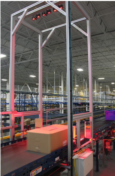
Cartons for retail store replenishment are scanned when passing through the scan tunnel.
