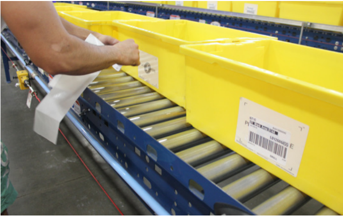
A bar code label is applied to the side of an order tote at the start of the piece pick process.
