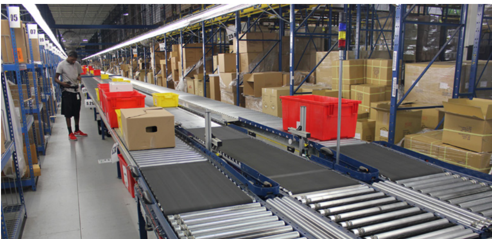
Piece picking occurs in the two level pick module.
