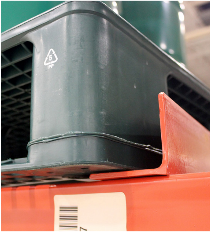
Pallet guides in the rack assure precise pallet placement for AGV pick-up at receiving.
