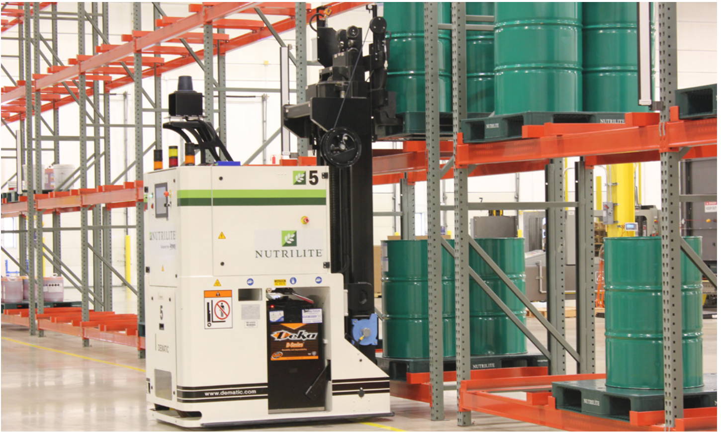
AGVs pick up pallets of inbound materials on one side of the pallet staging rack. Manual fork trucks drop off inbound pallets on the opposite side of the rack.
