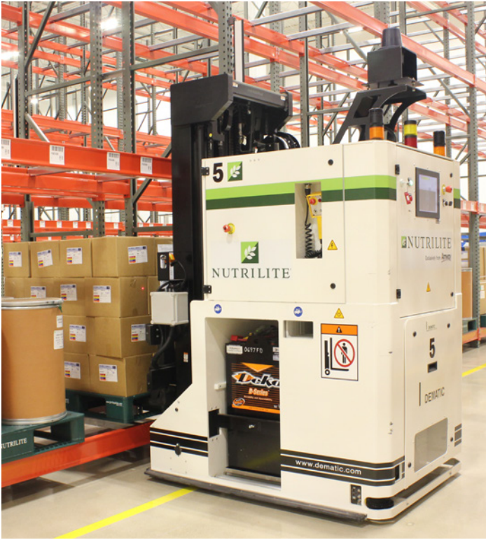
Production materials and finished products are stored in pallet racking by the AGV System.
