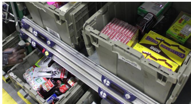
At the order assembly workstations, light-directed technology indicates the totes for operators to “put” the items. The slot display shows the quantities.
