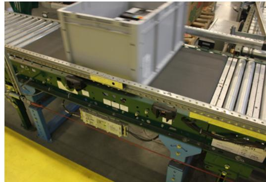
Each inbound inventory tote passes over an in-line weigh scale to confirm and verify stock keeping unit count.
