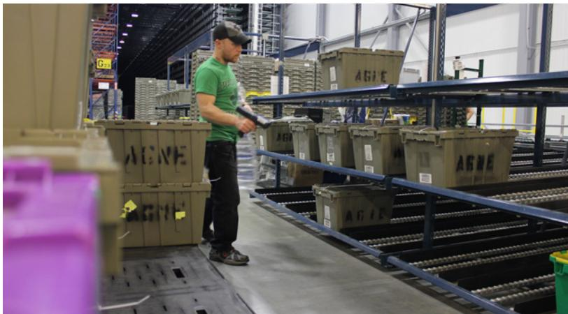
Completed order totes accumulate on flow rack structure. Operator scans each tote and is directed to appropriate pallet load.
