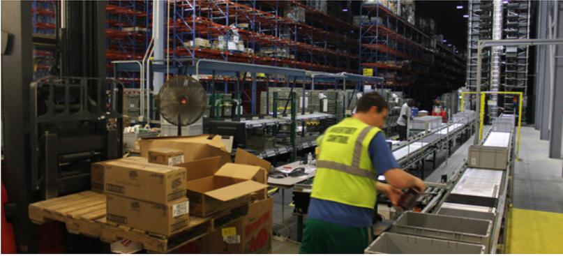
At the decanting workstation, each stock keeping unit is unpacked and transferred to an inventory tote.
