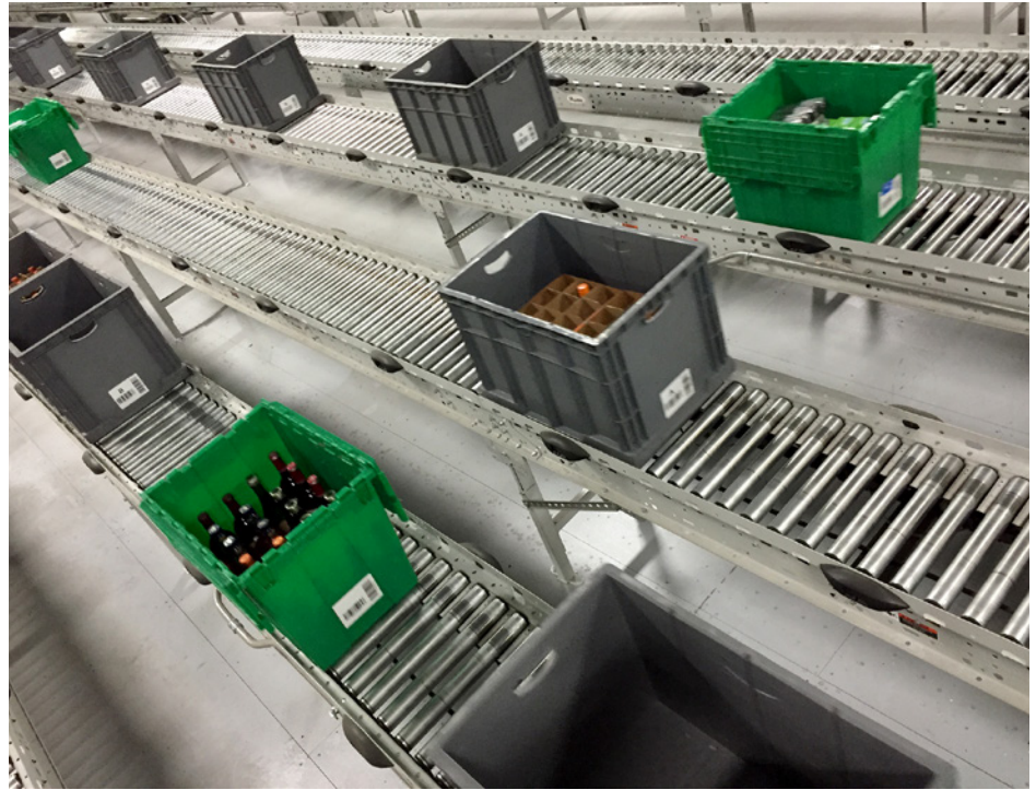
The convey and sort network is designed to accommodate the inventory totes (gray) and retail store totes (green). Transport of all totes between the functional areas of the distribution center is provided by the convey and sort network.
