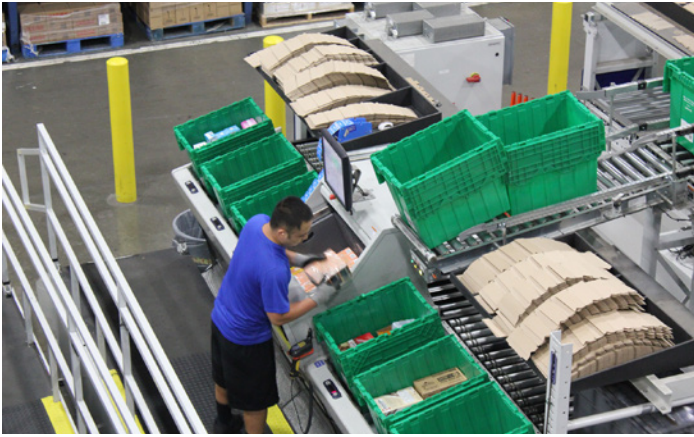
Good-to-person workstation allow six store totes to be assembled concurrently.
