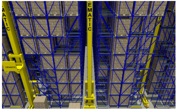
Load put-away logic is modeled for this pallet automated storage and retrieval system.
