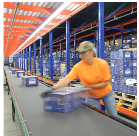
The system also accommodates case picking in a two level pick module
