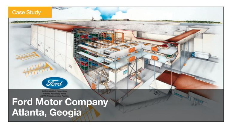
Ford's resequencing facility in Atlanta receives painted car bodies on skids from paint operations and delivers them in sequence to final trim. The loads are stored in the ASRS in the single deep position using only the rack locations that are between Storage and Retrieval Machines (SRM) aisles. If one aisle is taken out of service, all of the loads in that aisle can be accessed from the adjacent aisle using the SRM's double deep capacity.
