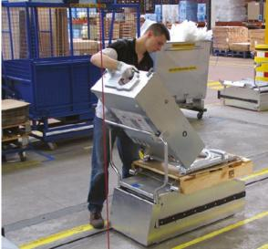
The level of the platforms is adjustable so that everyone can work at their ideal height. At the beginning of the line the units are placed diagonally, which permits easier assembly of the components. This has consequences for levels of absenteeism, which today are lower. And in order to keep the assembly work varied, the assemblers are regularly swapped between work posts.
