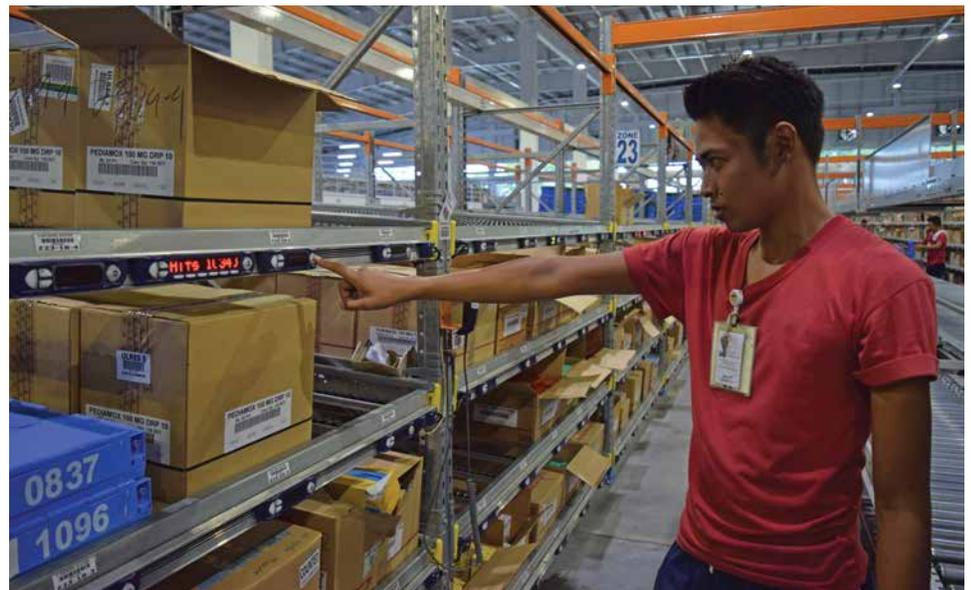
Stock locations in the PTL system are fitted with a digital readout indicating the quantity of items to be picked for each order, enhancing accuracy.
