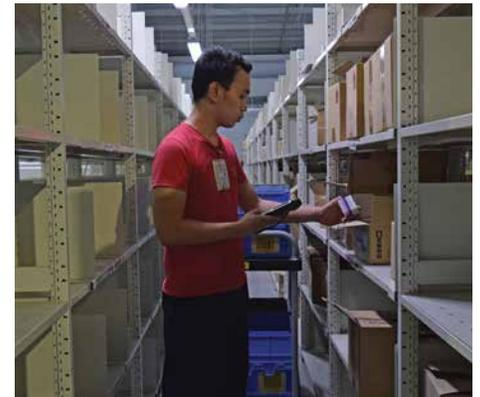
Orders typically commence on the Mezzanine Floor where slower moving SKUs are located, with pickers using lightweight, hand-held wireless mobile computing terminals for picking.
