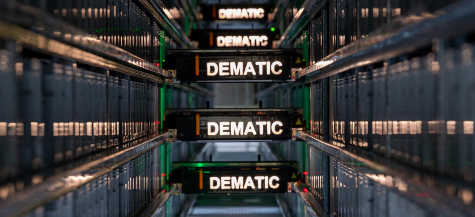
As part of the solution, Dematic set up a Dematic Multishuttle® automated storage and retrieval system. Products are placed in open totes, which are then stored in high-density racks. The system selects the best storage locations and shuttles automatically transport the incoming totes to designated rack locations. These towering racks reach the ceiling of the main storage floor, maximising the storage density of the warehouse.
