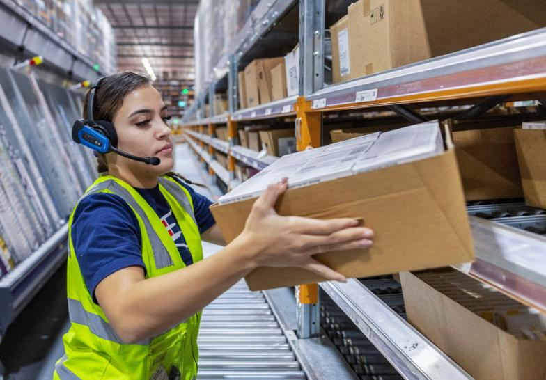
“The Dematic GTP Picking Solution delivers items directly to workstations – eliminating the need for operators to manually locate and retrieve items by travelling across the DC floor. The solution enhances operator performance by combining high-density, secure storage with the rapid rates and accuracy of directed picking from the ergonomically designed workstations,” said Darren Rawlinson, Dematic’s Regional Solutions Development Director, APAC.
