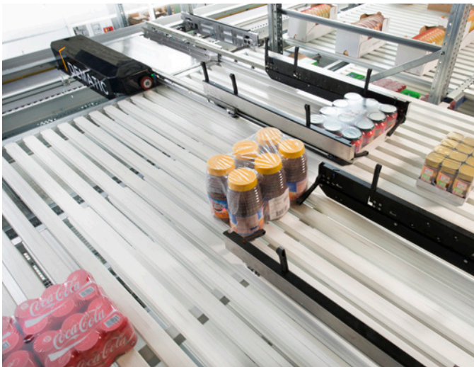
The Multishuttle module supports transfer of cases between aisles. This process, called inter-aisle transfer, optimizes system performance.
