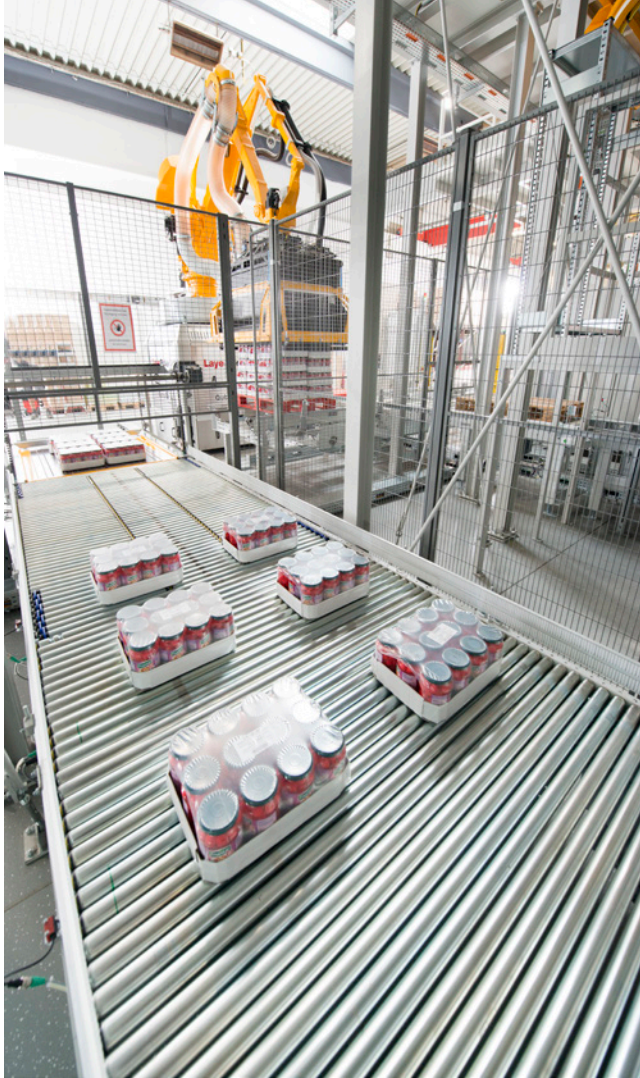
Depalletizing is accomplished using a delayering robot.
