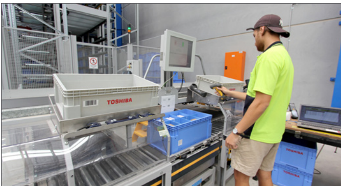
Modular workstation presents inventory tote (blue tote on lower conveyor) to worker. Items are picked to gray totes above.
